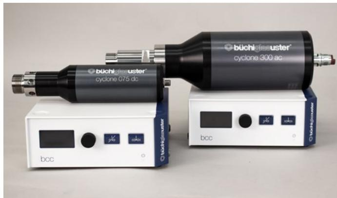
cyclone 075 and cyclone 300 magnetic stirrer drives for pressure ranges from full vacuum to high pressure
